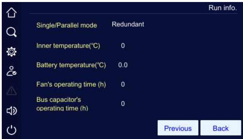
Working status page 2 (parallel UPS)
