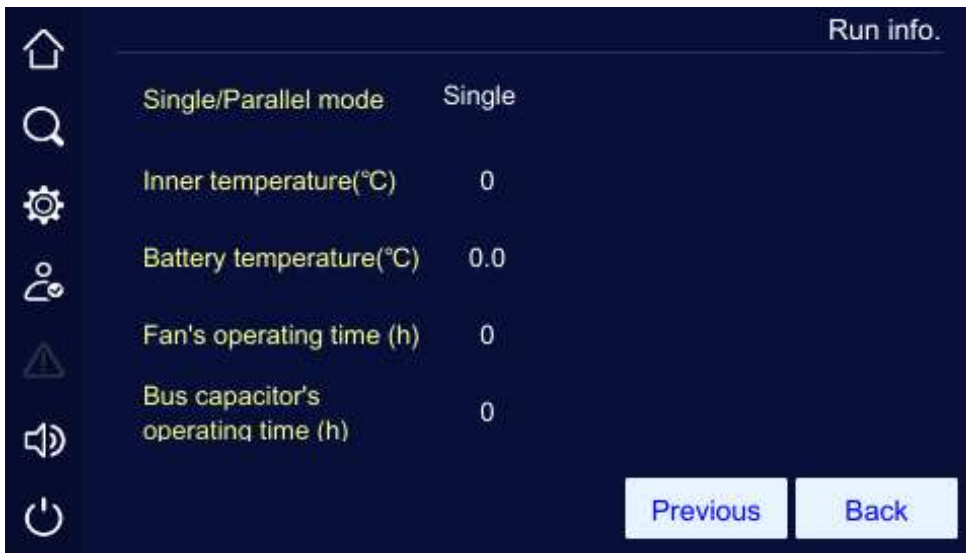
Working status page 2 (single UPS)
