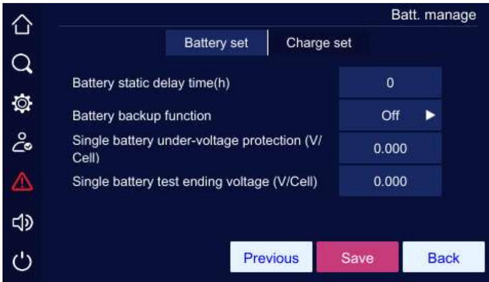
Battery set page 2 of battery management
