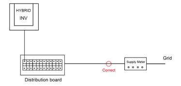
If there has been installed an inverter or AC coupled energy storage system already, the first please ensure they can not be wired into distribution board, then the new hybrid system and CT install positions are as below.
