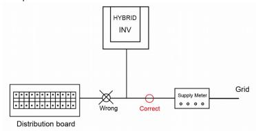
• If the inverter is wired in the distribution board, the CT install position is as below.
