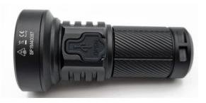
**SPERAS M4** is powered by a lithium battery in 18350 format, present in the sales package. The 6A 1100mAh battery is protected and rechargeable via the USB-C port on the M4. It takes about 2 hours and 10 minutes to complete the charge (0.9A).
